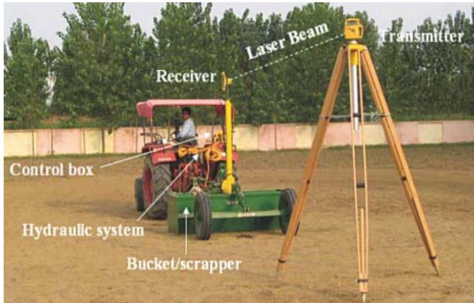
**Fig. 1.15 : Working mechanism of laser leveler**
