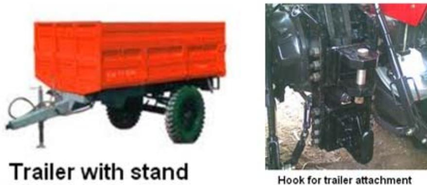
**Fig. 1.16: Two wheel trailer and hook for trailer attachment**
